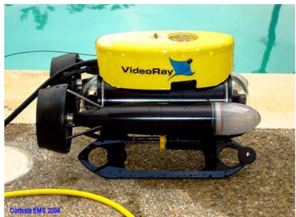
1. *This equipment represents a considerable increase in safety as it does not involve submerged personnel, who are therefore no longer susceptible to nitrogen saturation which could lead to decompression, as well as making greater use of the working day.*
